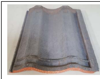
Photo 5 Concrete Tile—Bottom View
