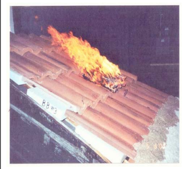
Photo-1 showing the most heat affected area on the surface of the Concrete Roof Tile
